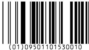
Figura 5.5.2.1.1-1. GS1 DataBar Omnidirectional
