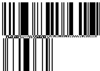
Figura 5.5.2.3.2-1. Simbolo GS1 DataBar Expanded Stacked
