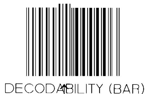
Figura 5.12.5.12-1 Calibration symbol with engineered low decodability grade
