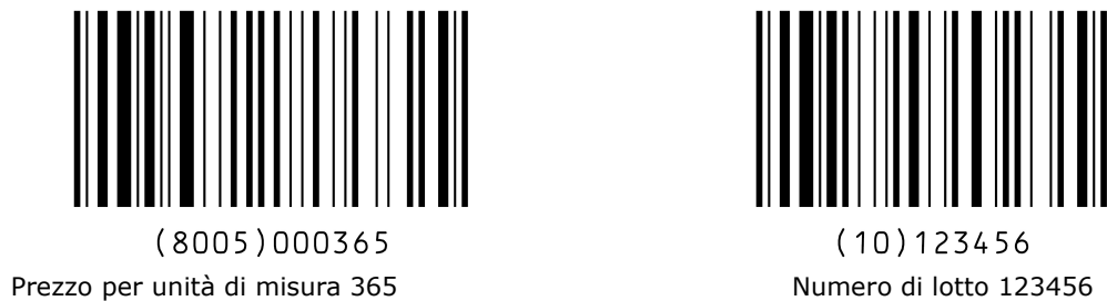
Figure 7.8.6.2-2. Data encoded in one concatenated GS1-128 symbol
