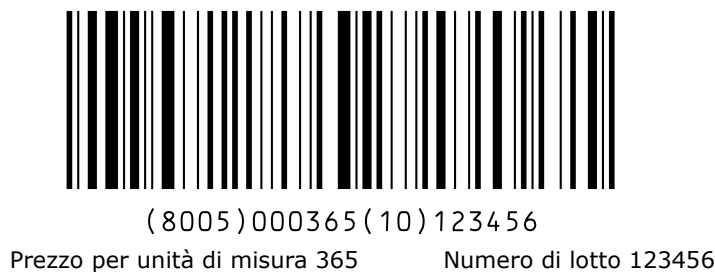
Figure 7.8.6.2-2. Data encoded in one concatenated GS1-128 symbol
