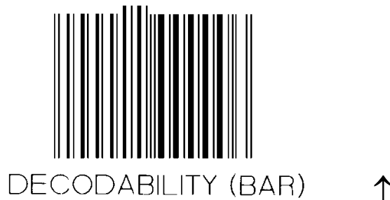
Figura 5.12.5.12-1 Calibration symbol with engineered low decodability grade
