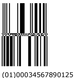
Figura 5.5.2.1.4-1. GS1 DataBar Stacked Omnidirectional
