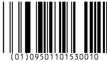
Figura 5.5.2.1.1-1. GS1 DataBar Omnidirectional
