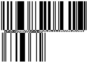
Figura 5.5.2.3.2-1. Simbolo GS1 DataBar Expanded Stacked
