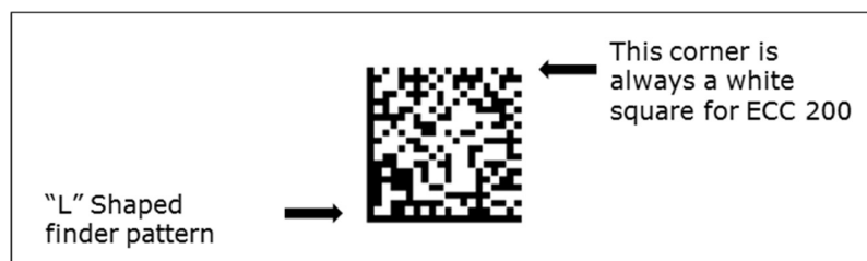
Figure 5.6.2-1. GS1 DataMatrix symbol
