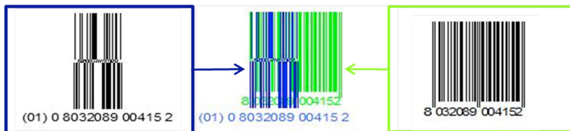
Figura 1.2: Confronto GS1 DataBar Omnidirectional Stacked – EAN-13
