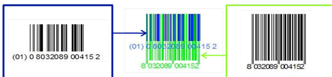
Figura 1.1: Confronto GS1 DataBar Omnidirectional – EAN-13
